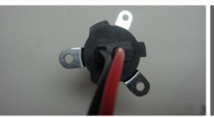
Secure the plugn-play harness to the stock headlamp wiring harness location. Make sure that the red ballast wire goes to the driver's side ballast.
