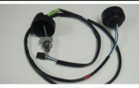
Press the metal bulb holder onto the HID bulb. Make sure the base of the metal makes contact with the HID bulb base
